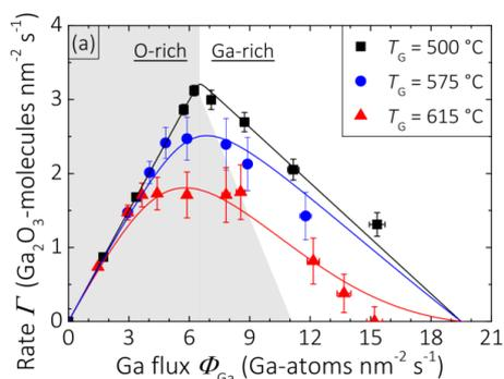
Fig. 1: The growth rate of  $\text{Ga}_2\text{O}_3$  as function of the Ga flux for different growth temperatures. The O flux was kept constant.
