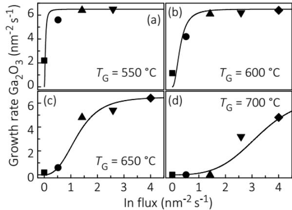
Fig. 4: (a)–(d) Dependence of the growth rate of  $\text{Ga}_2\text{O}_3$  on the In flux for different growth temperatures as indicated in the figures. Symbols represent experimental data and solid lines are model predictions.[6]
