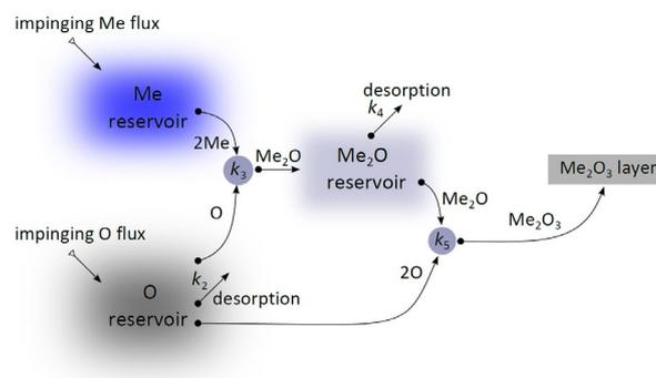
Fig. 2: Reaction scheme for  $\text{Me}_2\text{O}_3$  MBE ( $\text{Me}=\text{In, Ga}$ ), including all possible reactions occurring on the growth surface with reaction rate constants  $k_i$ .
