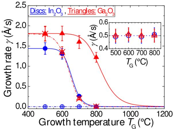
Fig. 3: Pseudo-binary growth rates of  $\text{In}_2\text{O}_3$  (discs) and  $\text{Ga}_2\text{O}_3$  (triangles) from the ternary compound  $(\text{In}_x\text{Ga}_{1-x})_2\text{O}_3$  as a function of growth temperature. The In-to-(In+Ga) flux ratio was set to 0.5. The impact of the (In+Ga)-to-O flux ratio  $r_{\text{Me}}$  is demonstrated by different symbols: filled (O-rich,  $r_{\text{Me}}=0.5$ ), crossed (Me-rich,  $r_{\text{Me}}=2.0$ ), and inset: highly O-rich,  $r_{\text{Me}}=0.1$ .
