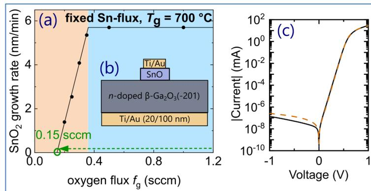
Figure 1: (a) Finding the right growth conditions for SnO based on in-situ measurements of the growth rate of SnO<sub>2</sub>. (b) Schematics of the processed, vertical SnO/Ga<sub>2</sub>O<sub>3</sub> *pn*-diode. (c) Current-voltage characteristics of the diode including fit (orange, broken line) to the diode equation. The inset indicates the low turn-on voltage.
